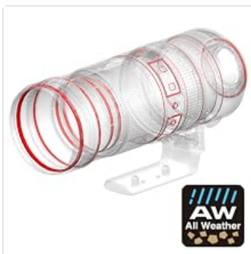
Figure 6: Diagram highlighting the All Weather (AW) sealing points for dust and moisture resistance.
