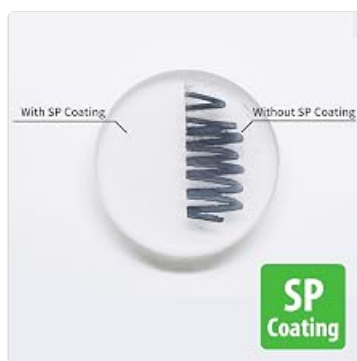
Figure 5: Illustration demonstrating the effectiveness of Super Protect (SP) Coating against dirt adhesion and for easy wipe-off.
