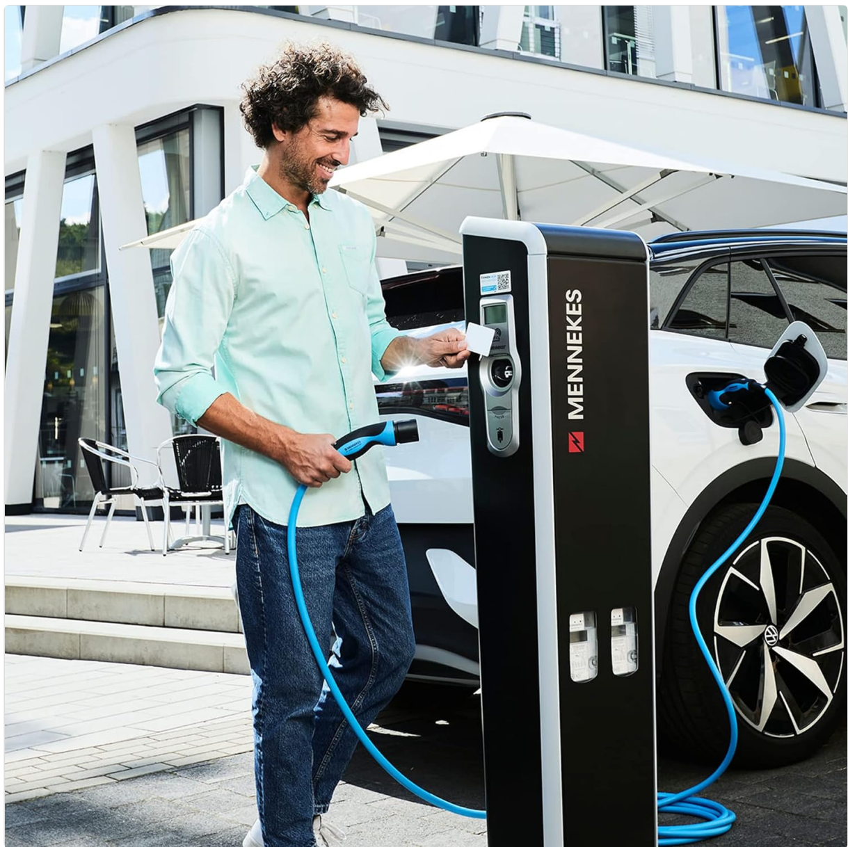
Image: A user connecting the Mennekes Type 2 charging cable to an electric vehicle at a public charging station, demonstrating the connection process.
