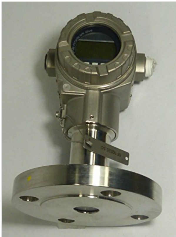
Figure 3.1: Front view of the Endress Hauser Cerabar PMC71 pressure transmitter. This image shows the robust metallic housing, the display window, and the process connection flange at the bottom.
