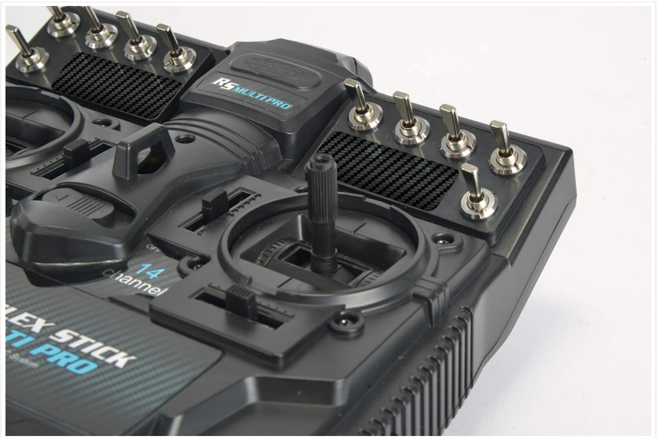
Figure 5.1: Detail of the transmitter's control sticks and various switches for proportional and switching functions.
