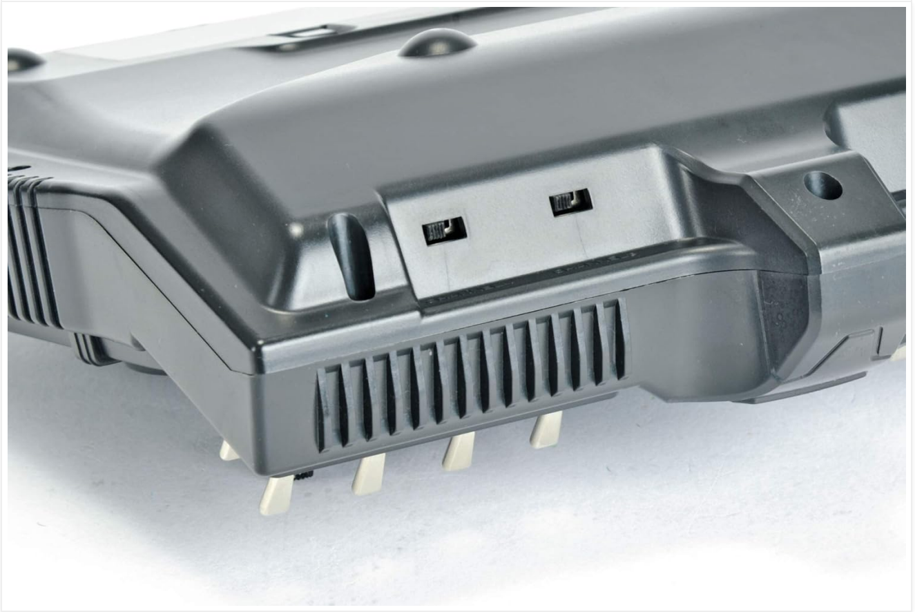
Figure 4.1: Rear view of the transmitter, indicating the location for battery installation and the Graupner-J/R charging socket (positive pole inside).
