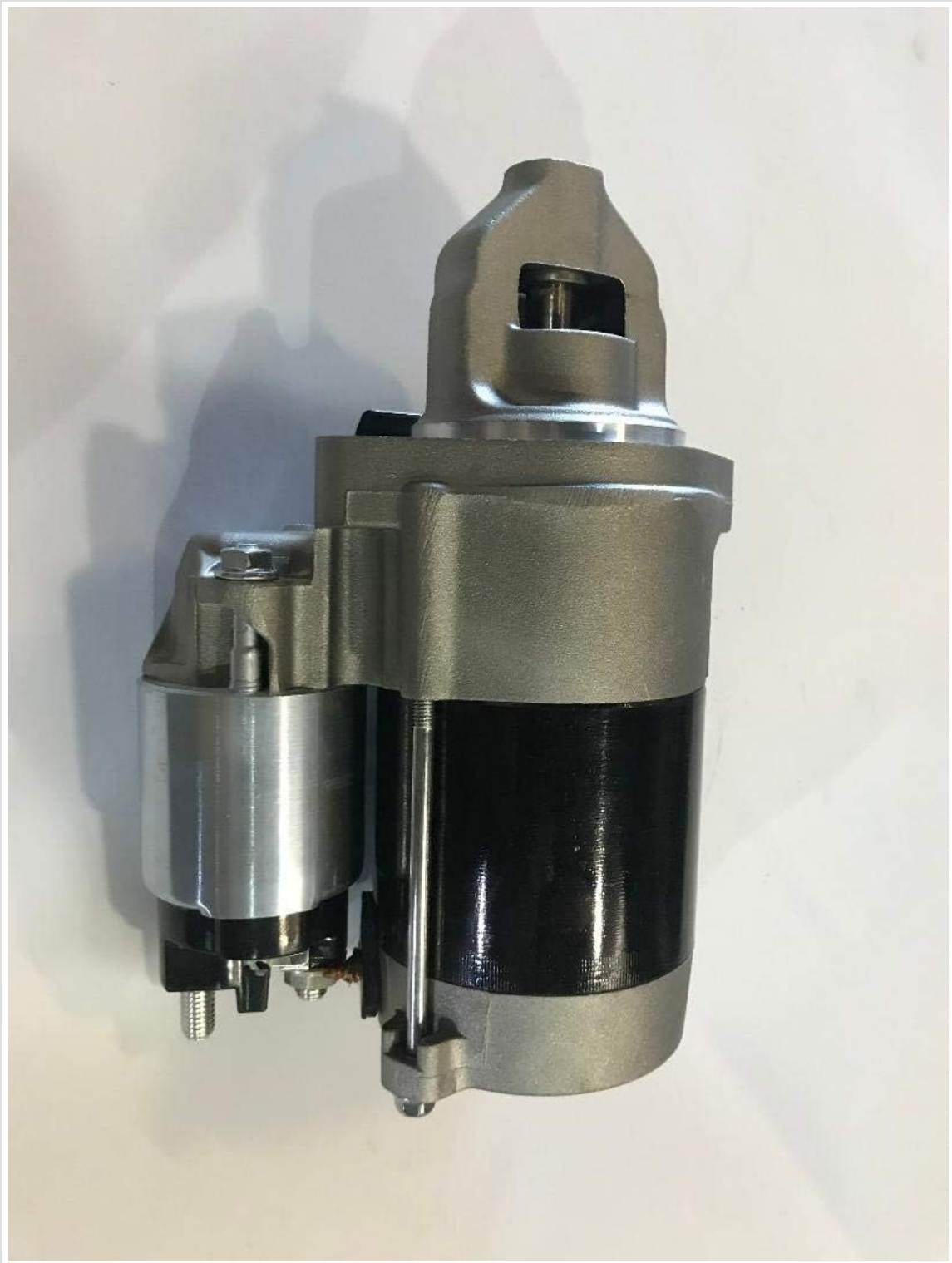
Figure 3: Rear view of the starter assembly, highlighting the mounting points and the motor housing. This view assists in proper alignment during installation.
