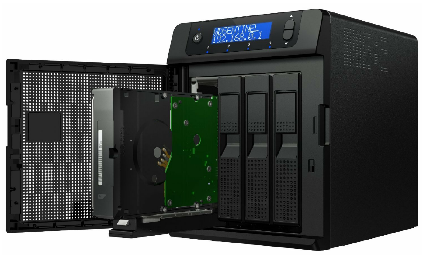
Figure 3: Illustrates the easy hot-swap capability of a hard drive in the WD Sentinel DX4000.
