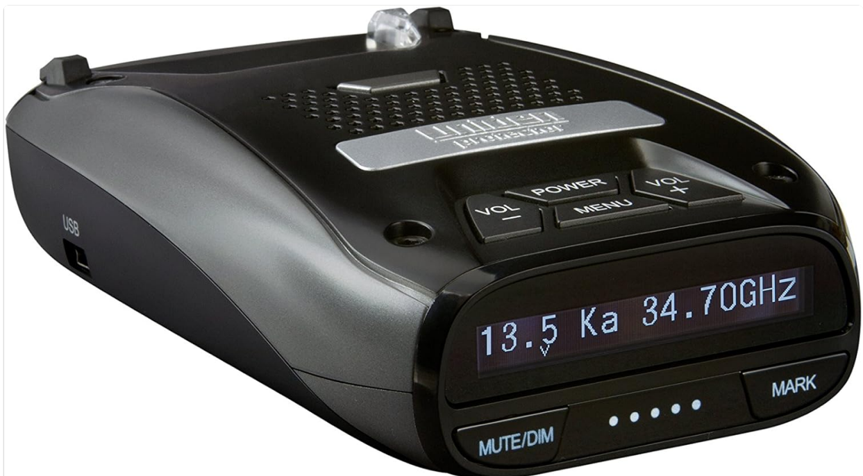
Figure 3.2: Angled view of the Uniden LRD950, illustrating the top-mounted control buttons (Power, Vol+/-, Menu) and the
