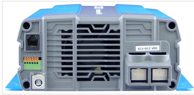
Image: Rear panel of the inverter, highlighting the DC input terminals (42.0-66.0 VDC) and the cooling fan. Connect battery cables here.
