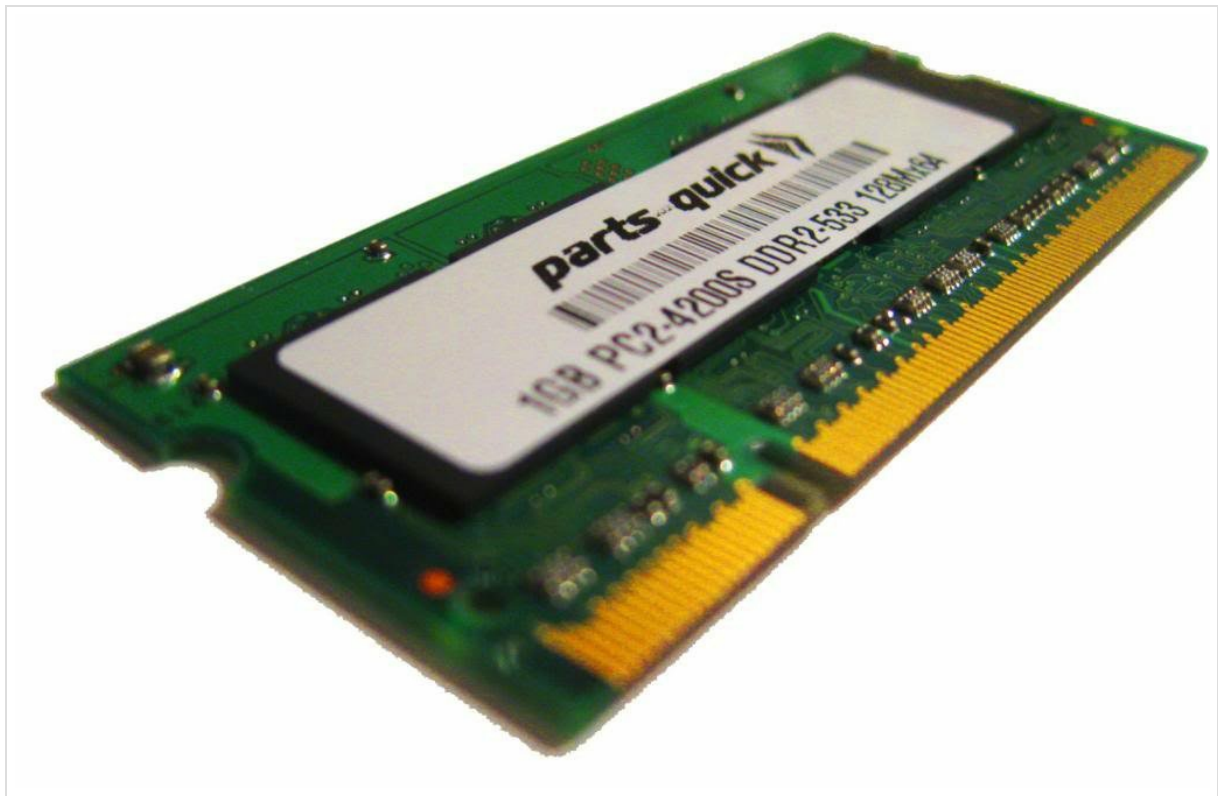
Figure 3.1: A close-up view of the PARTS-QUICK 1GB DDR2 PC2-4200 SODIMM RAM module, showing the green circuit board, memory chips, and gold-plated connectors.
