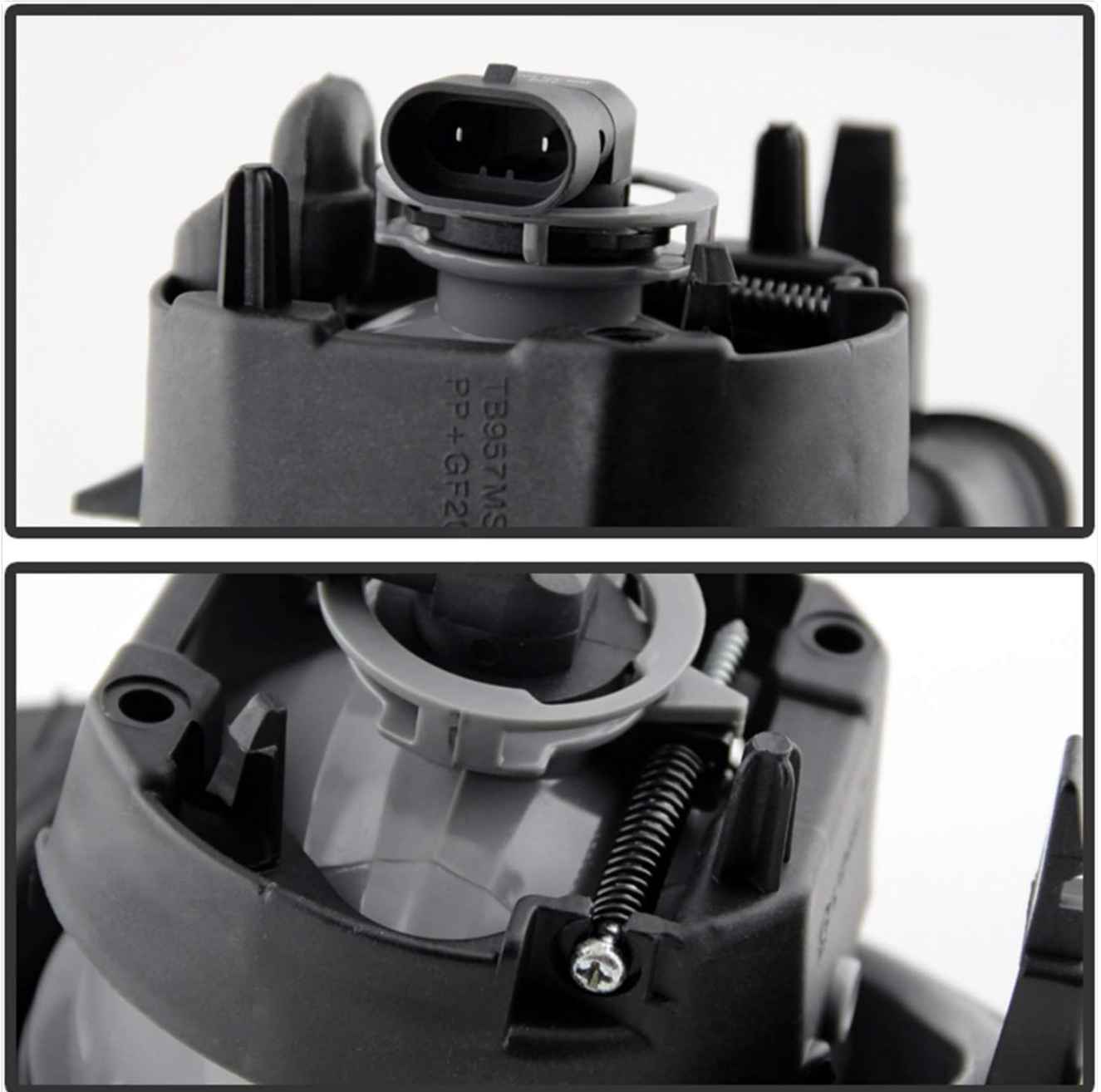
Image 4.2: Close-up of the electrical connector and the adjustment screw for beam alignment on the fog light unit.
