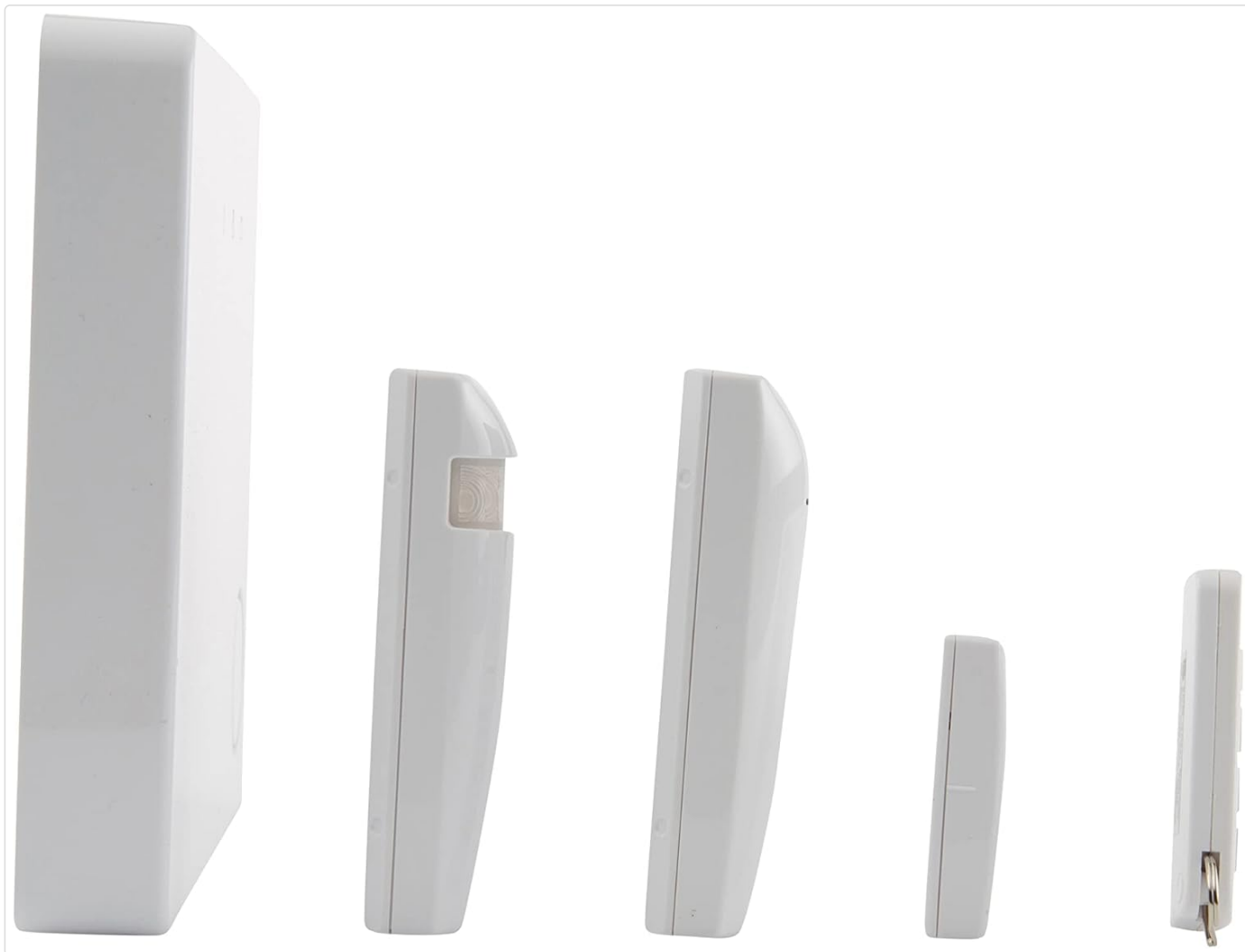
Figure 4.2: Side view of the Smartwares HA701IP alarm system components, showing the central unit, motion sensor, magnetic contact, and remote control, highlighting their compact design.
