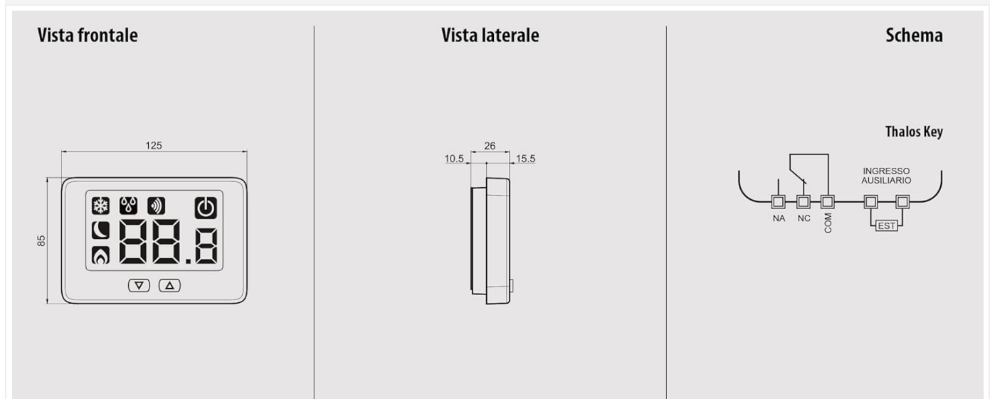
Figure 2: Installation diagram illustrating the front dimensions, side profile, and wiring schematic for the VEMER THALOS Key Thermostat.
