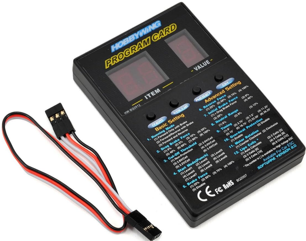
Image: A detailed view of the HOBBYWING LED Program Card, highlighting the 'ITEM' and 'VALUE' displays, along with the control buttons for programming.
