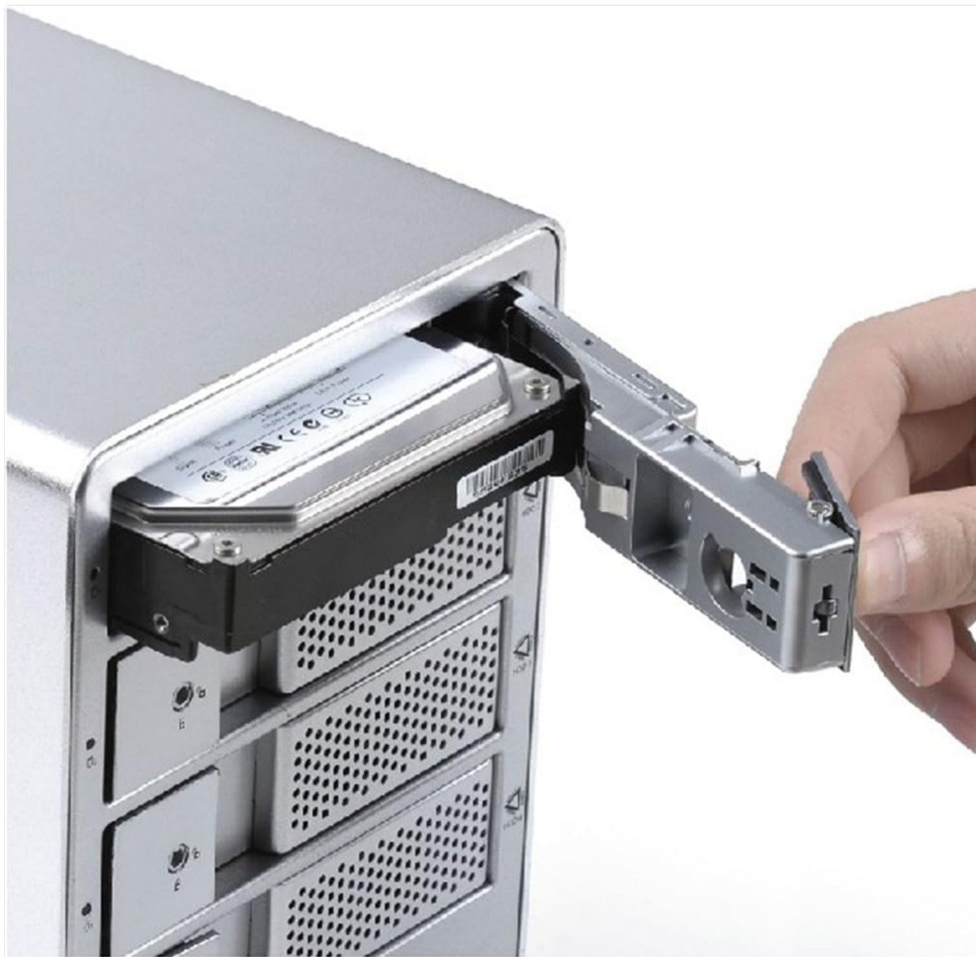
Image: Close-up of hard drive installation.
