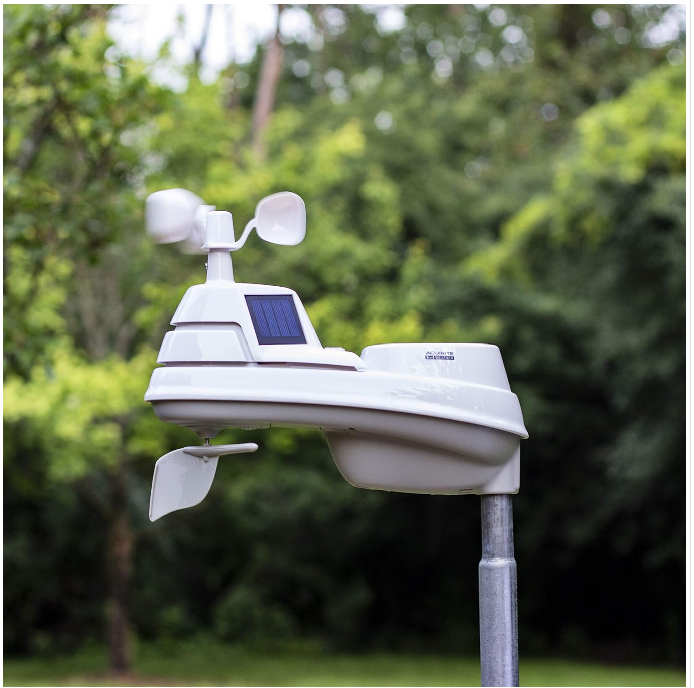
The weather sensor mounted on a pole in a backyard, demonstrating typical outdoor placement.
