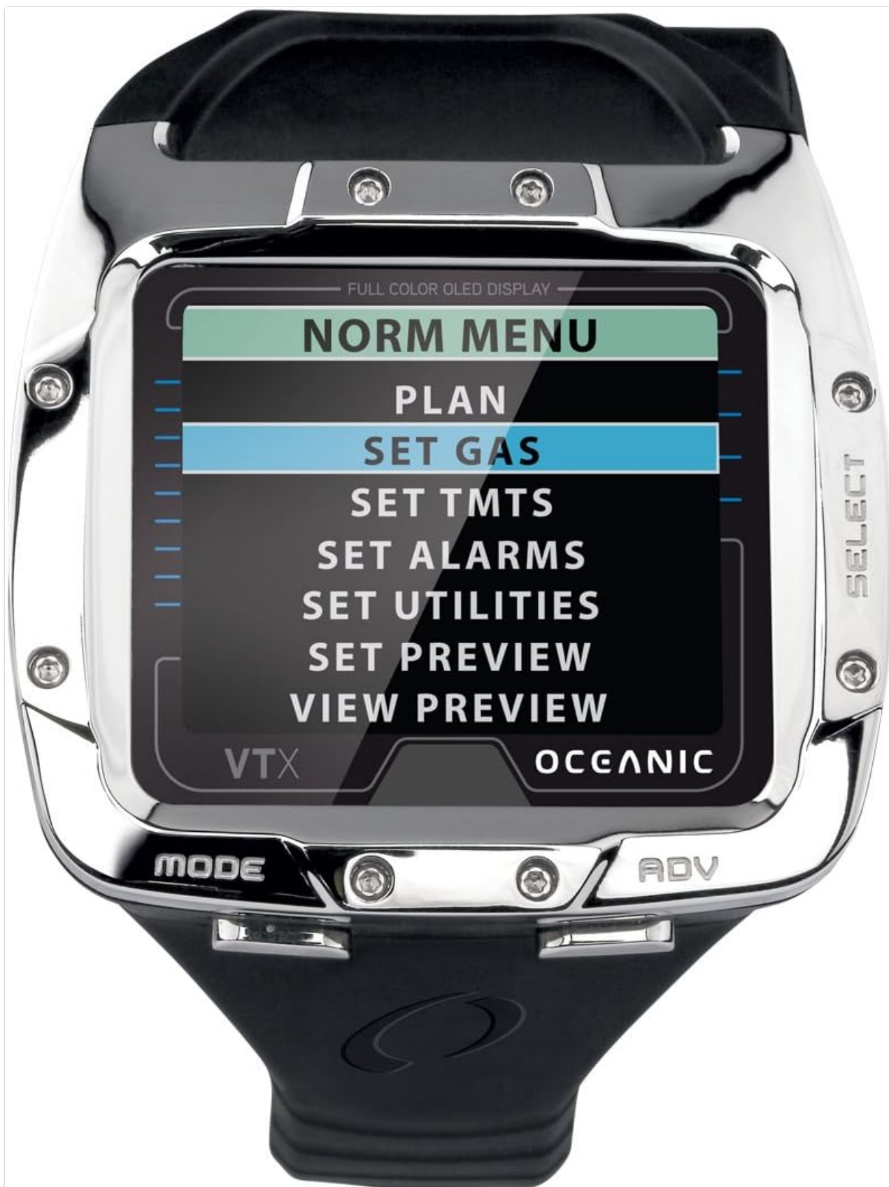
Image: The VTX display showing the 'NORM MENU', which is used for initial setup and configuration of dive parameters.
