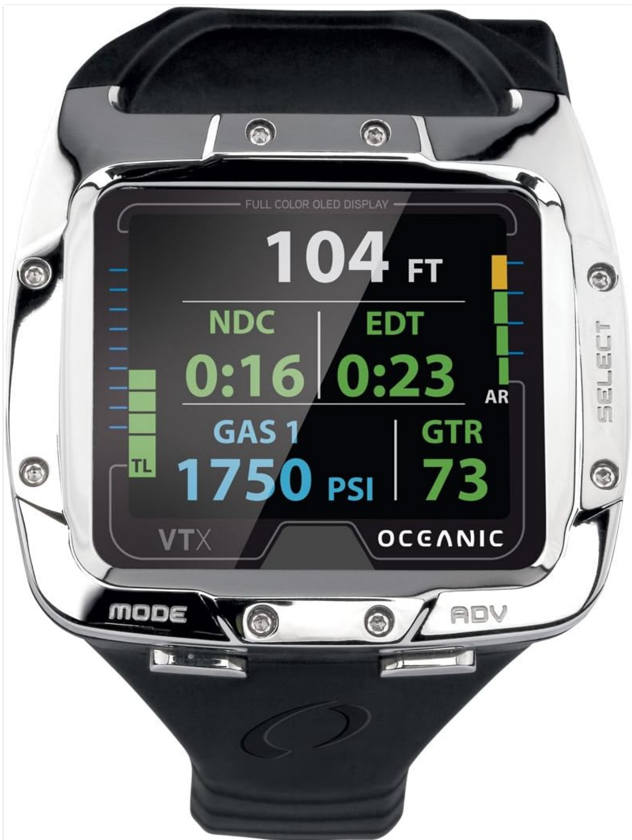
Image: The VTX display showing current depth (104 ft), No Decompression Limit (NDC), Elapsed Dive Time (EDT), Gas 1 pressure (1750 PSI), and Gas Time Remaining (GTR).
