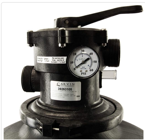
Figure 5.1: Pressure Gauge Detail. This close-up image shows the pressure gauge mounted on the 7-way valve. Monitoring this gauge is essential for determining when backwashing is required, typically when the pressure rises 8-10 PSI above the clean operating pressure.
