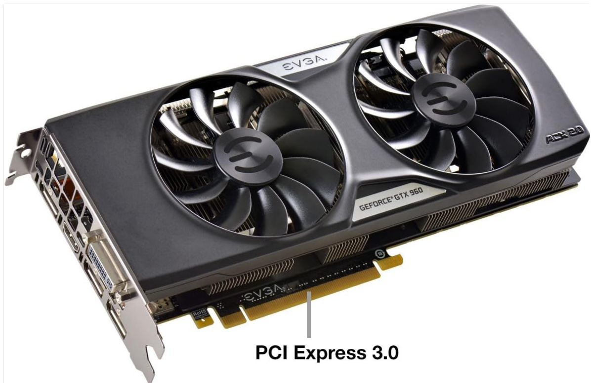
Image 3.1: The EVGA GeForce GTX 960 graphics card, highlighting its PCI Express 3.0 interface for motherboard connection.
