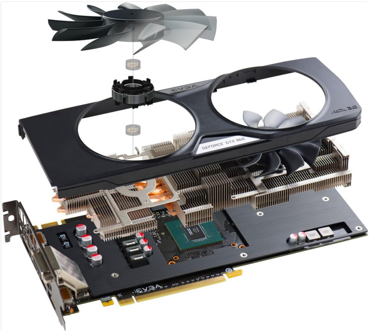
Image 2.2: Exploded view illustrating the components of the EVGA ACX 2.0 cooling system, including fans, heatsink, and PCB.
