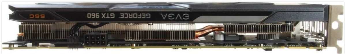
Image 3.2: Side view of the graphics card, indicating the location of the 6-pin PCIe power connector.
