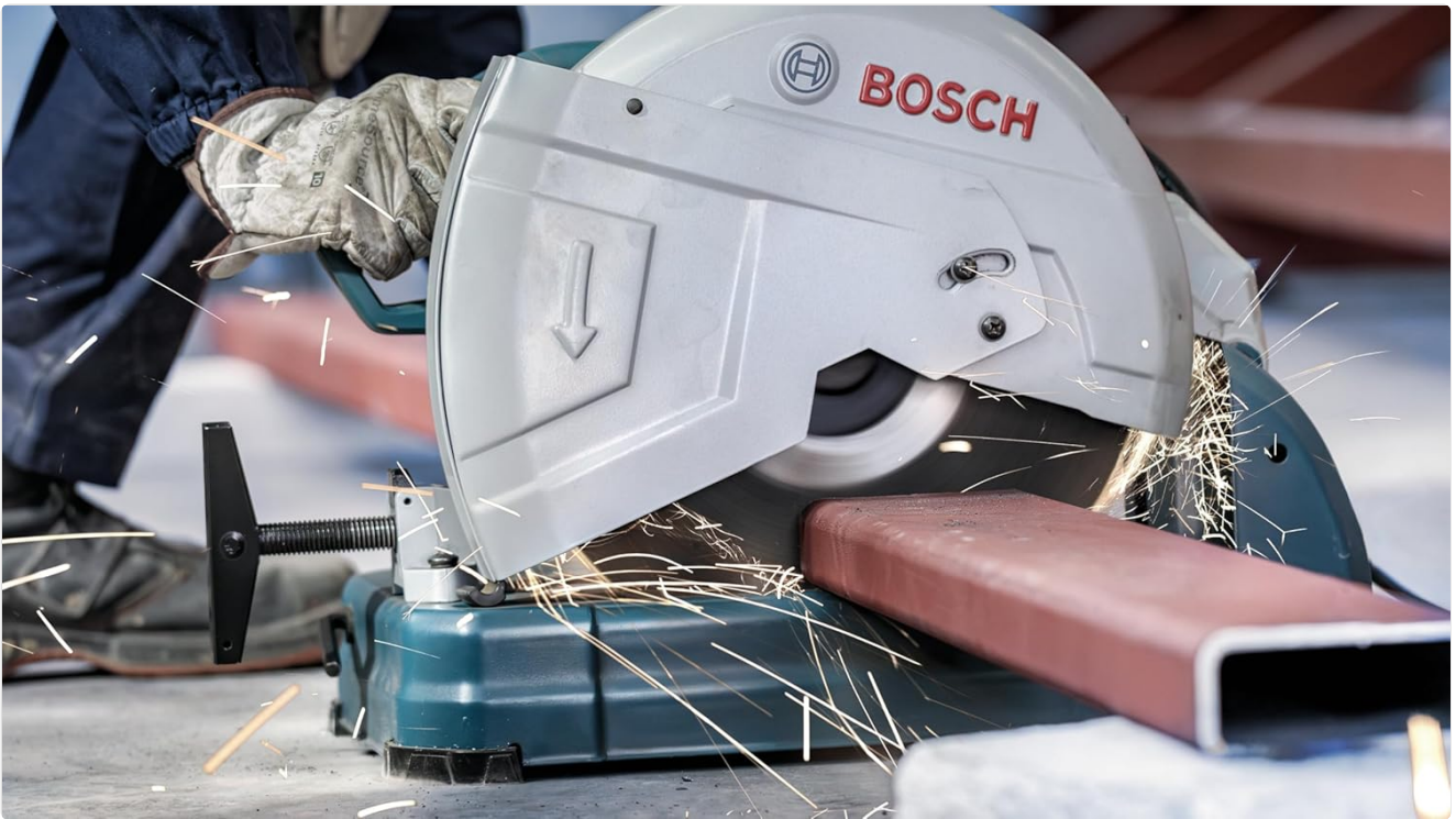
Image: The Bosch Expert for Metal cutting disc actively cutting a metal profile on a chop saw, demonstrating its primary function and the sparks generated during operation.
