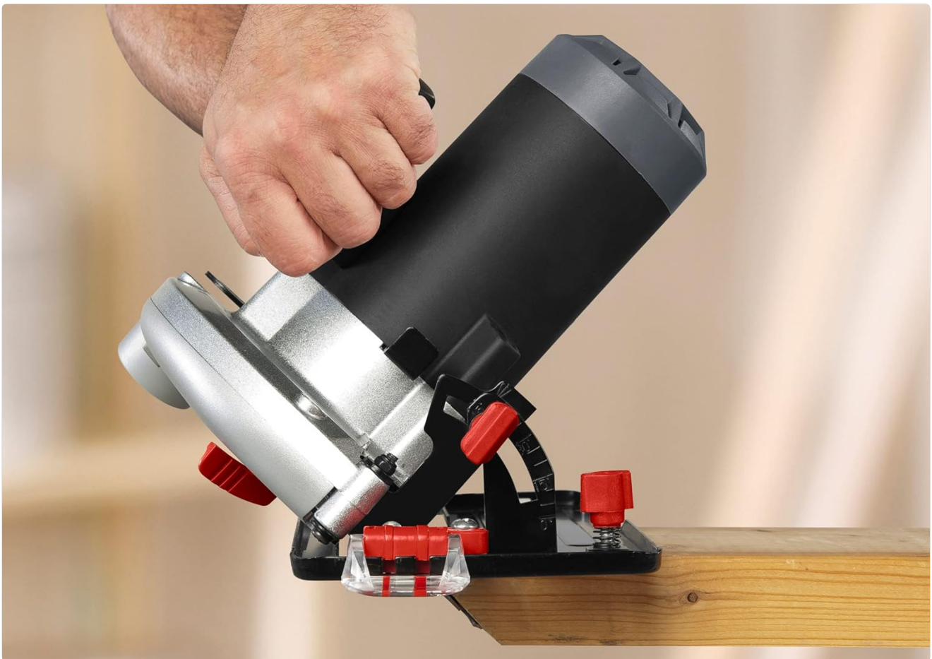
Figure 3.2: The circular saw adjusted for a bevel cut, demonstrating how the base plate tilts to achieve angled cuts up to 45 degrees.
