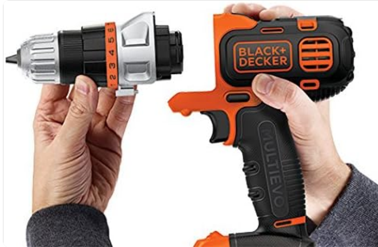
Figure 4.1: Illustrates the process of attaching or detaching an interchangeable head from the main multi-tool body, highlighting the secure connection mechanism.
