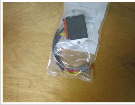
Image: The Wacker Neuson RT820 Voltage Regulator, shown here in its protective clear plastic packaging. The regulator unit is a metallic, rectangular component with a black heat sink on top, connected to a multi-colored wiring harness terminating in a gray connector.
