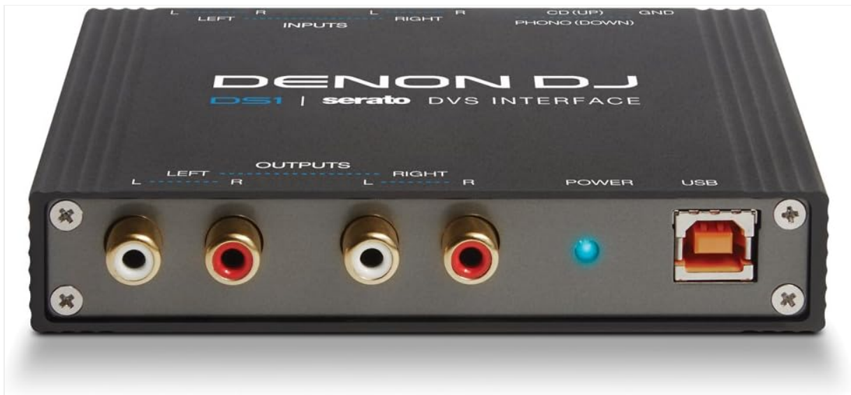
Figure 2: Front view of the Denon DJ DS1 interface with outputs and USB port.
