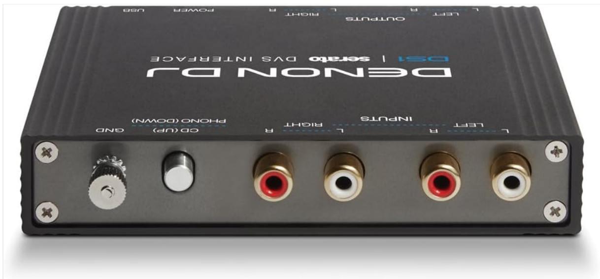
Figure 3: Rear view of the Denon DJ DS1 interface with inputs and ground terminal.
