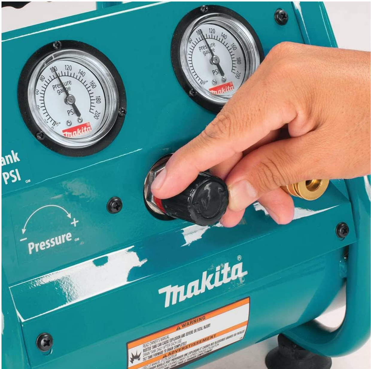
Figure 5: Adjusting the pressure regulator dial.
