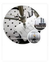
This image shows various product quality tests conducted by ATEN, including a keyboard life test, shock test, and drop test, ensuring product durability and reliability.
