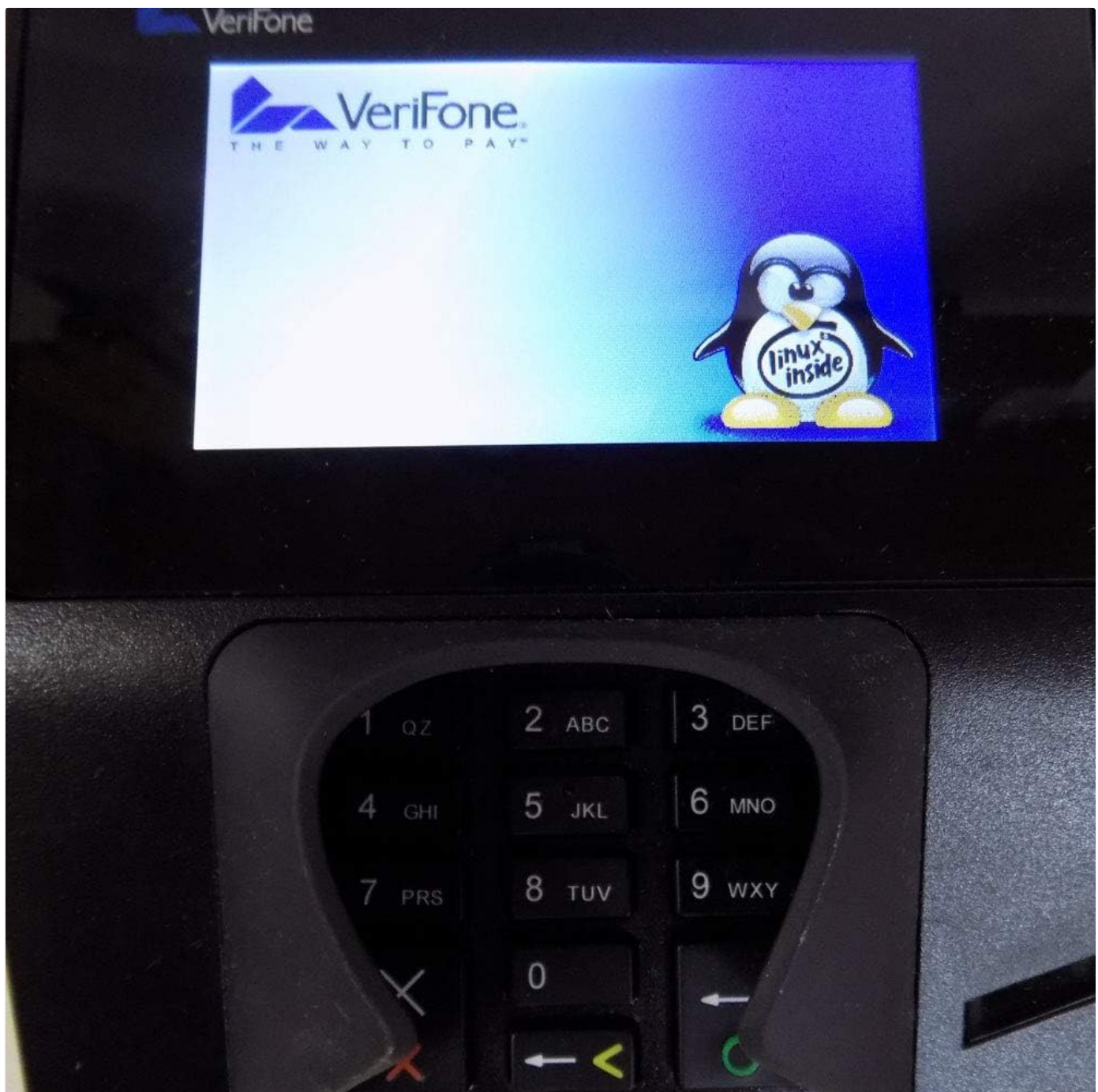
Figure 4.2: The VeriFone MX915 display during initial boot-up, showing the VeriFone branding and indicating its Linux-based operating system.
