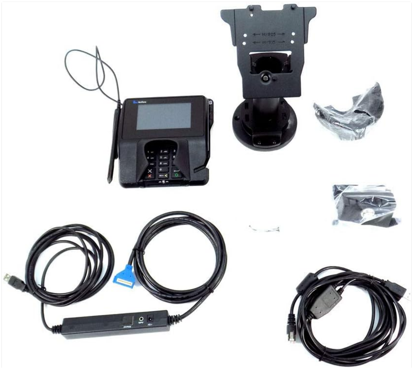
Figure 3.1: Contents of the Verifone MX915 package, including the terminal, stylus, various cables, and a mounting bracket. Please note that specific accessories may vary.
