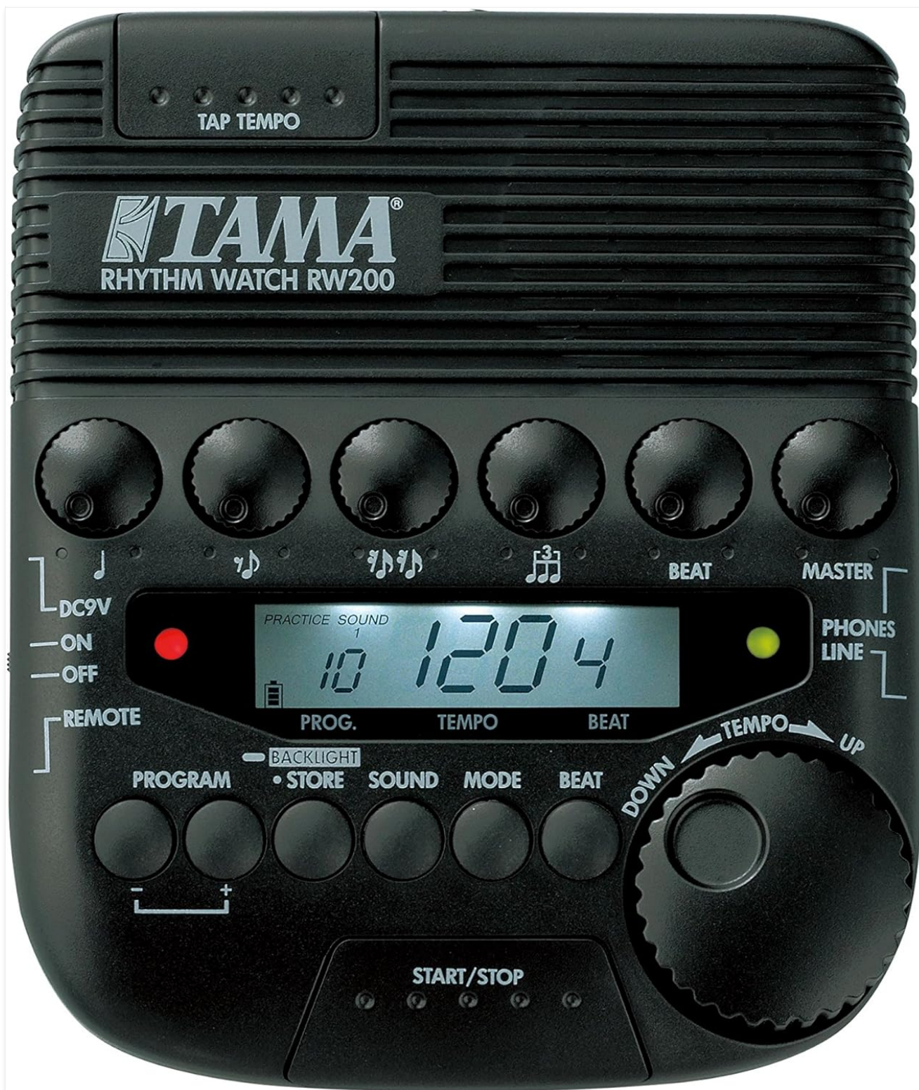
Figure 1: Front view of the Tama Rhythm Watch RW200, showing the main display, control knobs for sound and beat, program buttons, and the tempo dial.
