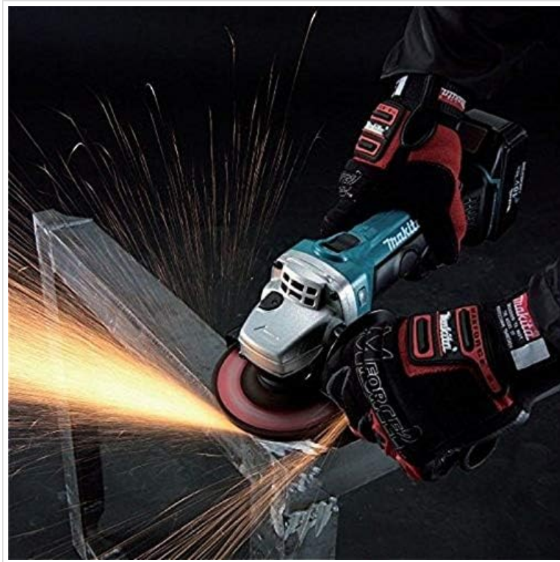
Figure 5: The angle grinder in action, demonstrating its use for grinding metal.
