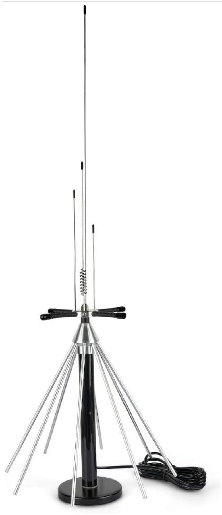
Figure 2.1: The Albrecht AE Desktop 1300 Scanner Antenna. This image displays the complete antenna assembly, including the central mast, radiating elements, and eight ground radials extending from the base, with the coaxial cable visible.
