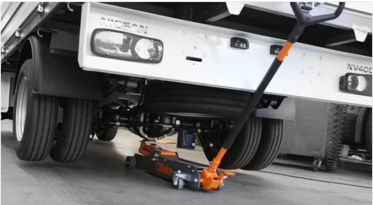
Figure 2: The Beta 30330030 Hydraulic Jack positioned under a vehicle's chassis for lifting. This demonstrates proper placement for vehicle elevation.
