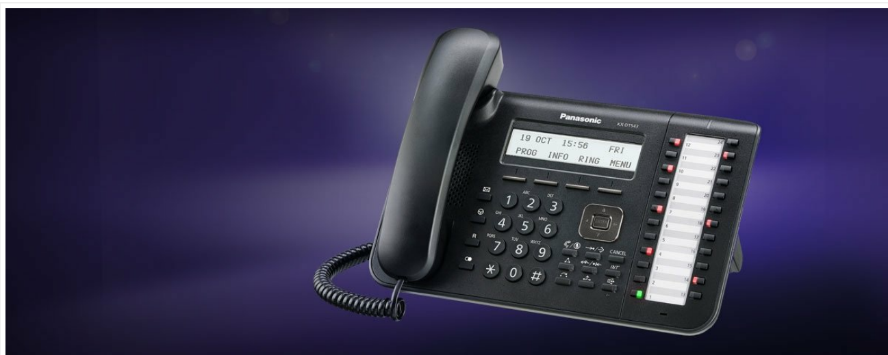
Figure 2.1: Panasonic KX-DT543 Digital Corded Telephone. This image displays the white model of the telephone, highlighting its 3-line LCD, keypad, and programmable function buttons.
