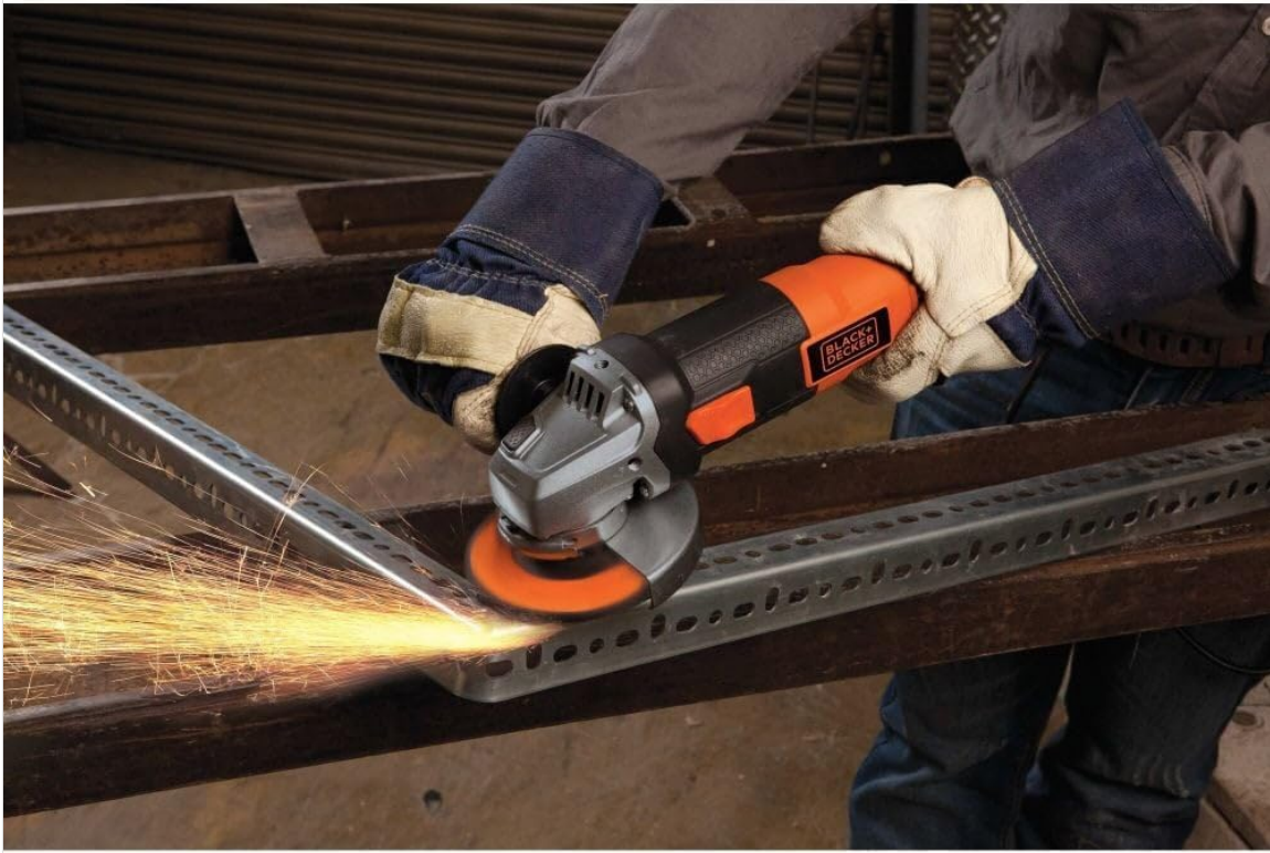
Image 5: The angle grinder being used for cutting metal, generating sparks.
