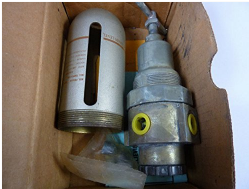
Figure 3: Components of the Air Line 26-1125-M3 Regulator, including the main body and the filter bowl.
