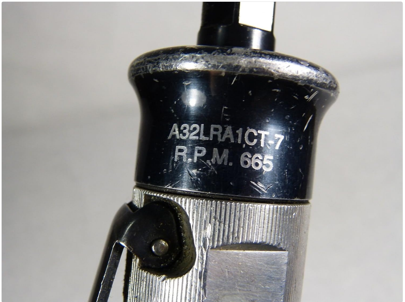
Figure 2: Close-up view of the tool's body, showing the model number A32LRA1CT-7 and the rotational speed (R.P.M. 665) clearly marked on the housing.
