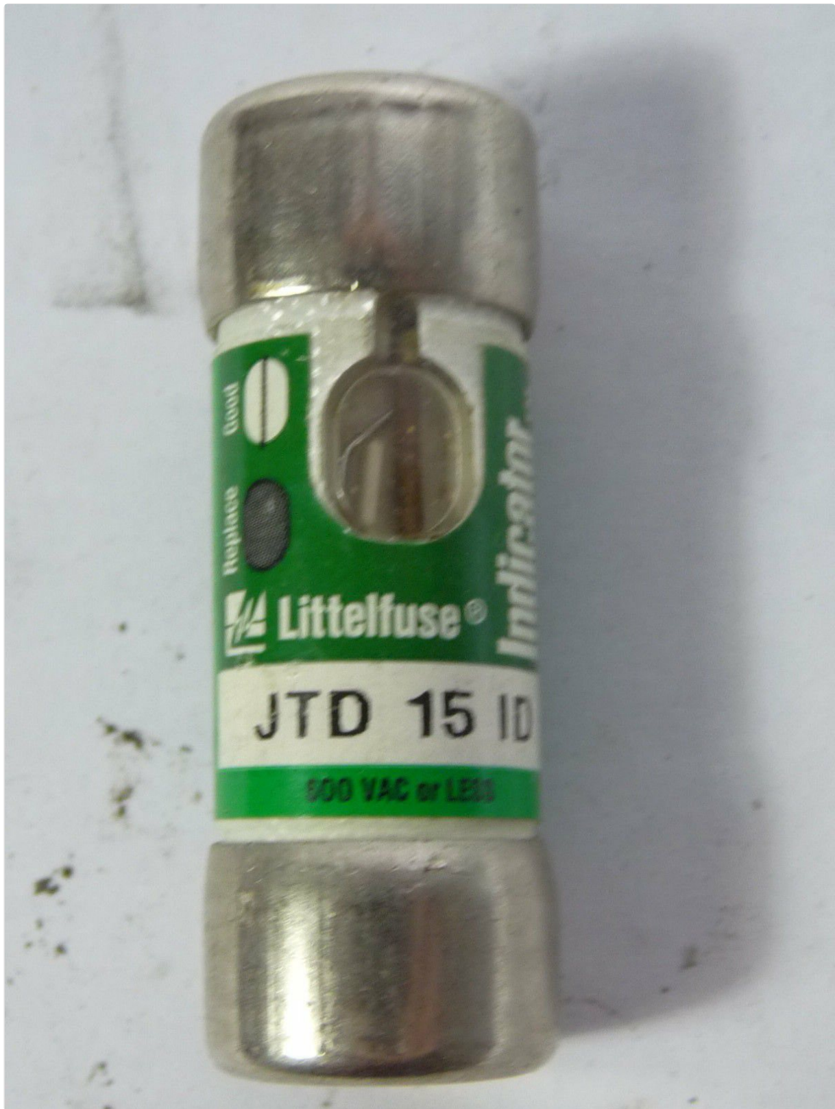
Figure 1: Front view of the Littelfuse JTD-15-ID fuse. The fuse is cylindrical with metal caps on both ends and a green and white label in the center. The label clearly shows "Littelfuse", "JTD 15 ID", and "Indicator". A small window on the label reveals the internal element and a "Good" or "Replace" indicator.
