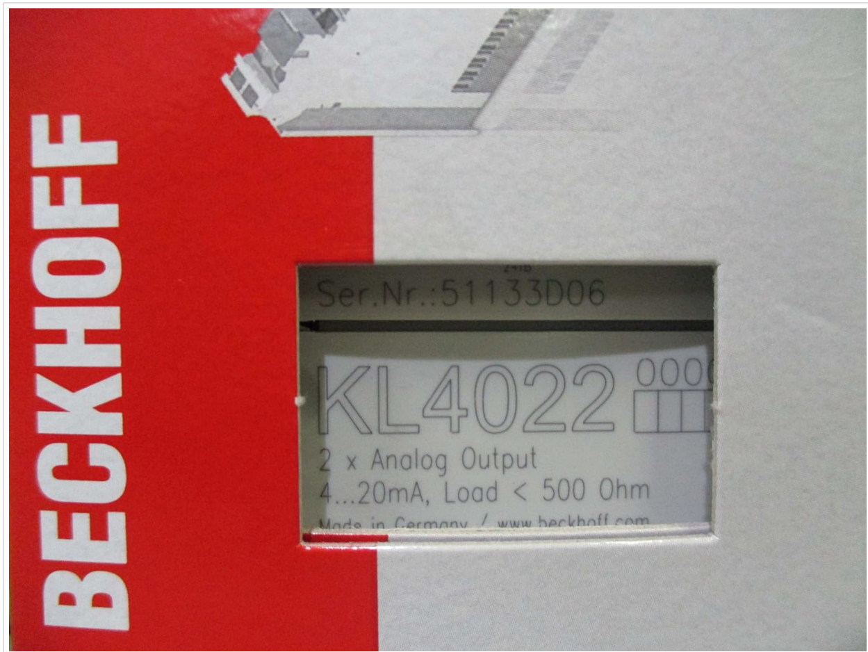
Figure 1: Front view of the Beckhoff KL4022 module packaging, displaying the model number and output specifications.
