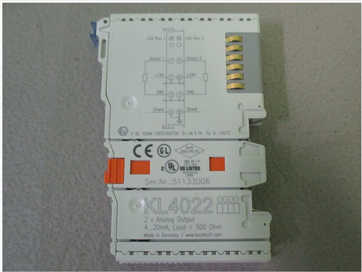
Figure 3: Detailed view of the KL4022 module, including its wiring diagram for analog outputs, power, and shield connections.
