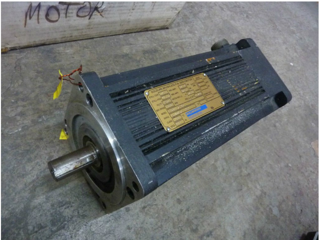
Figure 3.1: Full view of the Kollmorgen B-604-C-A3 Servo Motor, showing its robust industrial design.
