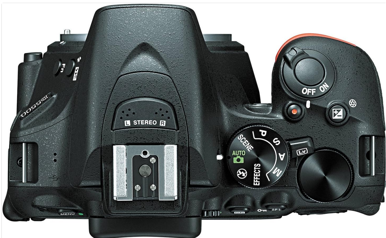
Figure 2: Top view of the Nikon D5500 camera, highlighting the mode dial with settings like P, S, A, M, Auto, Scene, and Effects. The power switch, shutter button, and command dial are also visible.
