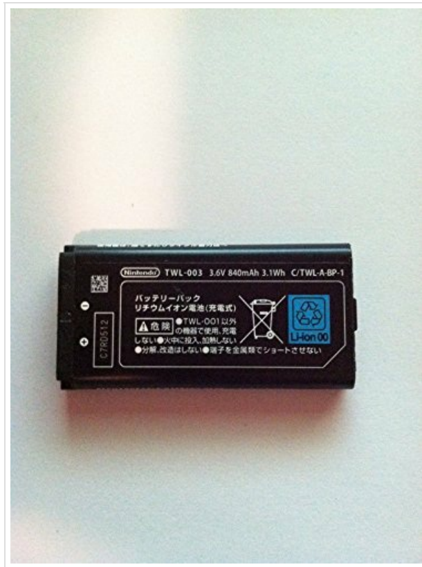
Figure 1: Nintendo TWL-003 840mAh DSI Battery. The label displays 'Nintendo TWL-003 3.6V 840mAh 3.1Wh C/TWL-A-BP-1' along with Japanese text and safety warnings, including symbols for recycling and not disposing of in regular waste.
