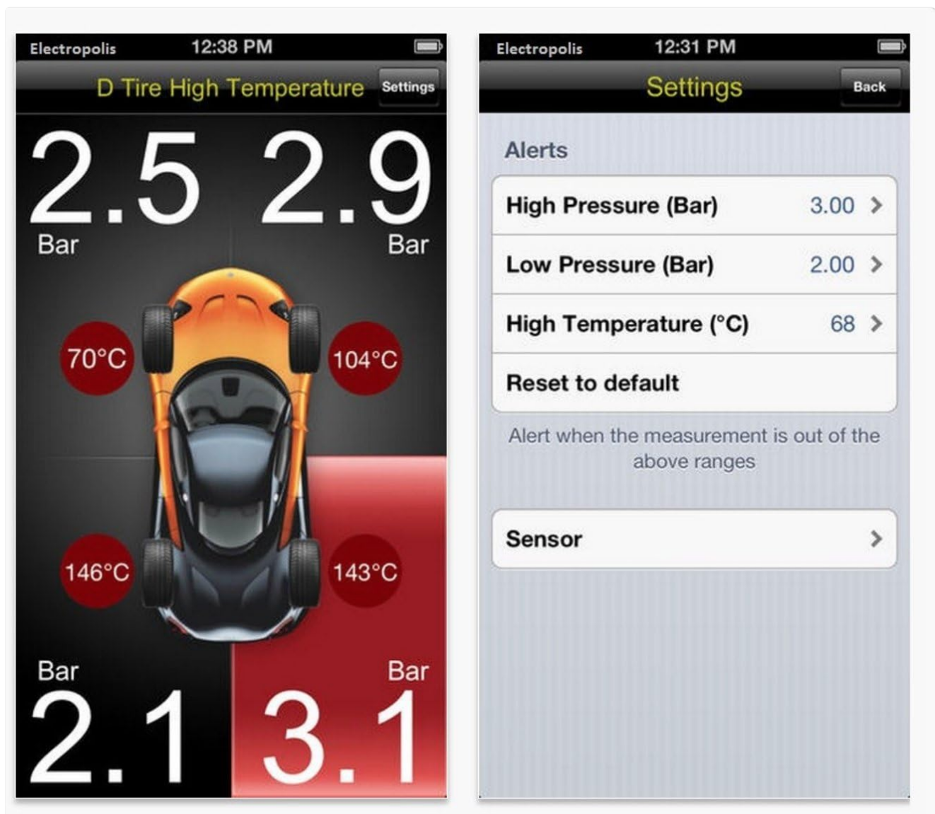
Image 3.3: A smartphone screen displaying the Spy TPMS application. The left panel shows real-time tire pressure and temperature, while the right panel illustrates the 'Settings' menu where alert thresholds can be configured.
