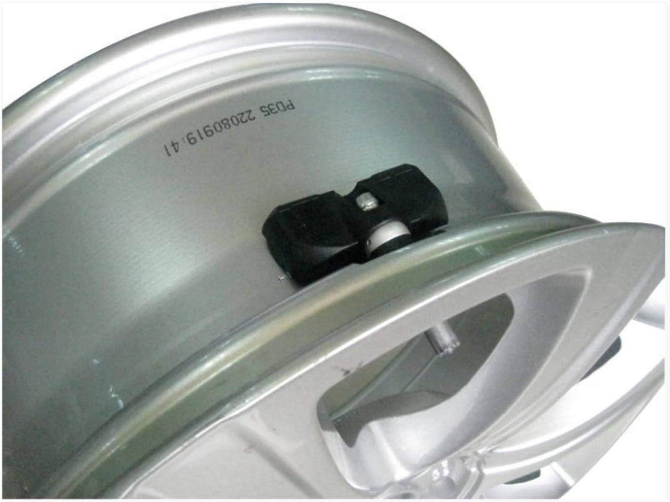
Image 3.1: A close-up view of an internal TPMS sensor correctly mounted inside a vehicle's wheel rim, illustrating its placement relative to the valve stem.
