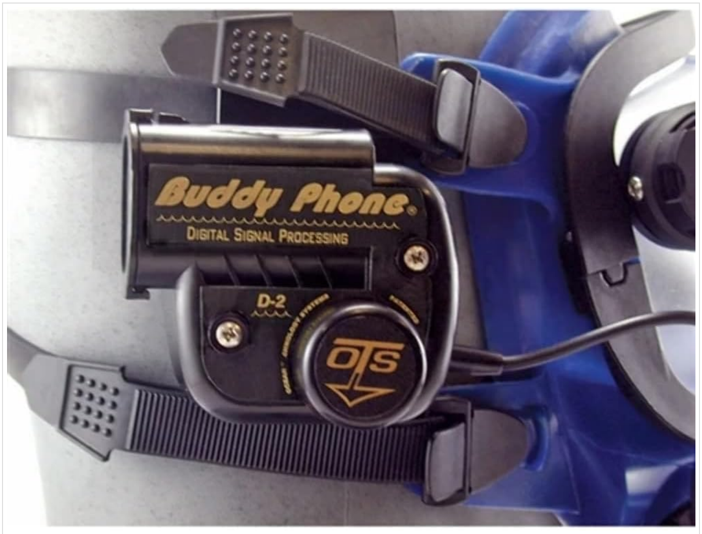
Image: The OTS Buddy Phone D-2 unit, labeled 'Buddy Phone Digital Signal Processing', is shown attached to the side of a blue full face diving mask. The unit features control knobs and a cable extending from it, indicating its connection to the mask's internal system. The attachment straps of the mask are visible, securing the communication device in place.
