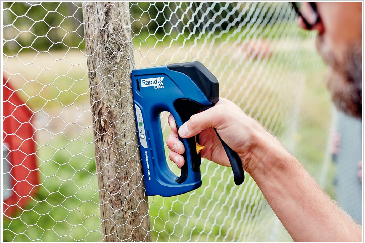
Figure 5: The Rapid ALU940 staple gun being used to secure wire mesh to a wooden fence post.
