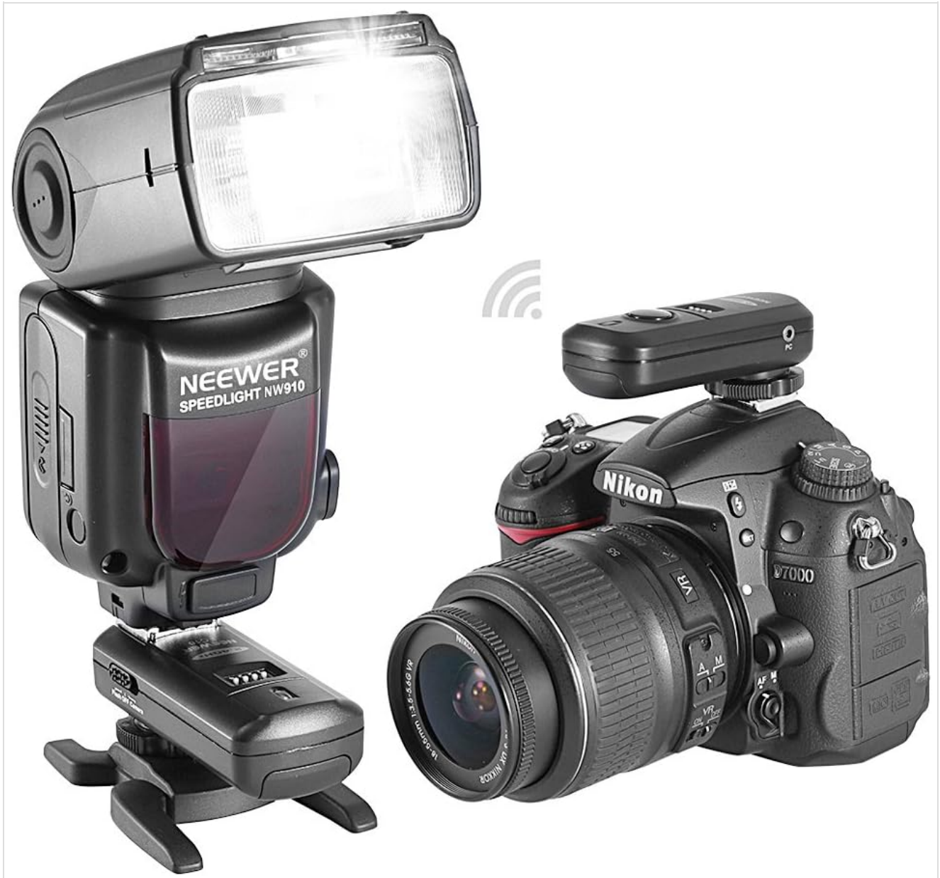
Figure 5.2: The Neewer NW910/MK910 Speedlite and the wireless trigger mounted on a Nikon DSLR camera for wireless flash operation.
