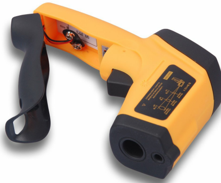
Figure 4: Battery compartment opened, showing terminals for 9V battery.
