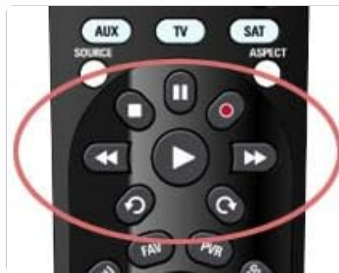
Figure 3: Close-up view of the media playback controls on the Shaw Direct IRC600 Remote Control, highlighted for easy identification.
