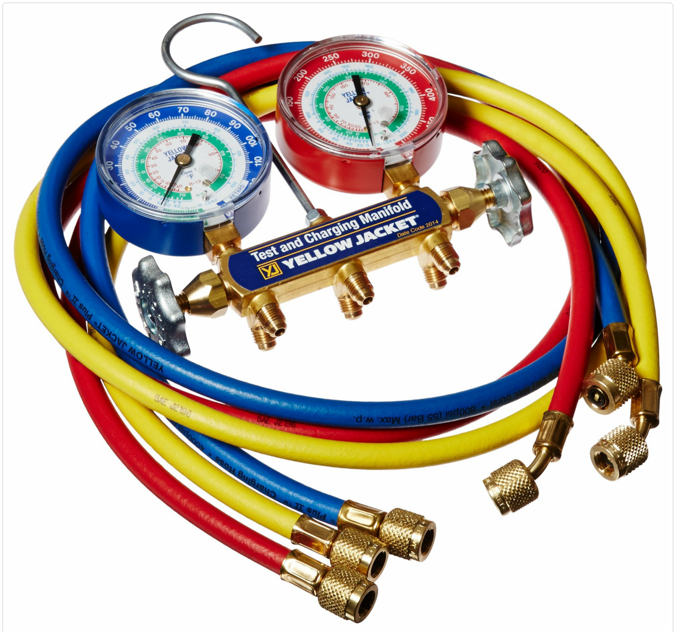
Figure 1: Yellow Jacket 42007 Series 41 Manifold Gauge Set. This image displays the central brass manifold, the blue low-pressure gauge, the red high-pressure gauge, and the color-coded blue, yellow, and red hoses with their respective fittings.
