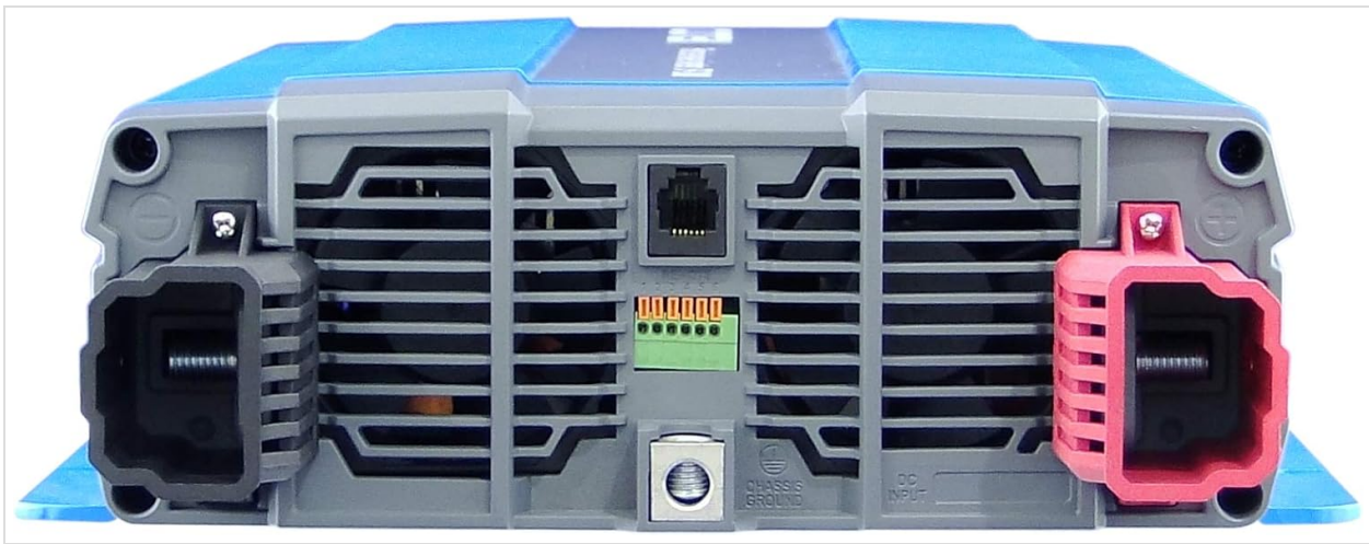
Figure 4.2: Rear view of the inverter, highlighting the DC input terminals (red for positive, black for negative), the chassis ground screw, and the remote control terminal.
