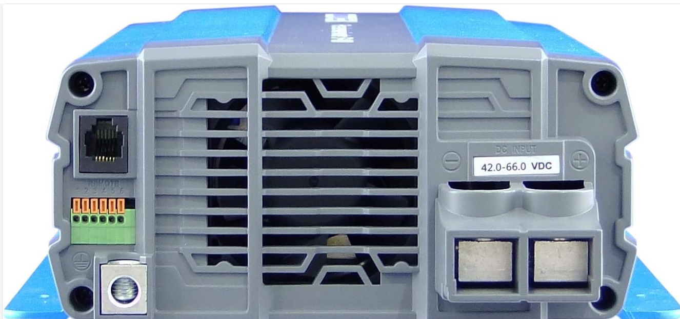
Figure 3.3: Rear panel of the inverter, showing the DC input terminals for battery connection, a remote control port (RJ45), and a green terminal block for remote ON/OFF control.
