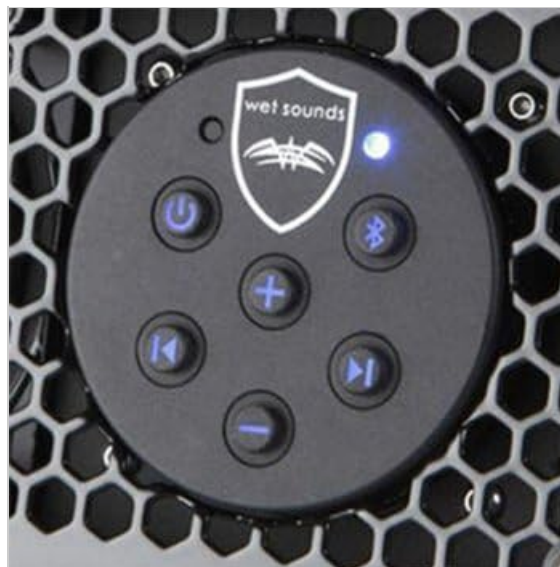
Figure 4.3: Close-up of the central control panel on the soundbar, showing power, Bluetooth, volume, and track control buttons.
