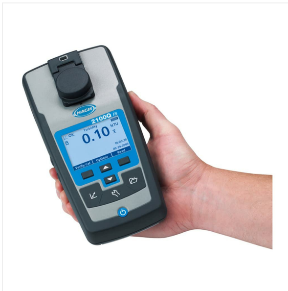
Figure 3.3: Close-up of the Hach 2100Q Turbidimeter display, showing a measurement reading and calibration status.
