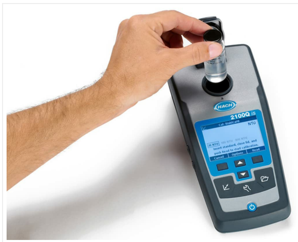
Figure 3.4: A user inserting a sample vial into the Hach 2100Q Turbidimeter's sample compartment for measurement.
